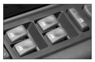
The controls for the power windows are located on the armrest on each of the side doors. The switches operate the windows when the ignition is in RUN, ACCESSORY or while Retained Accessory Power (RAP) is active. See *Retained Accessory Power (RAP)* on page 2-29.
